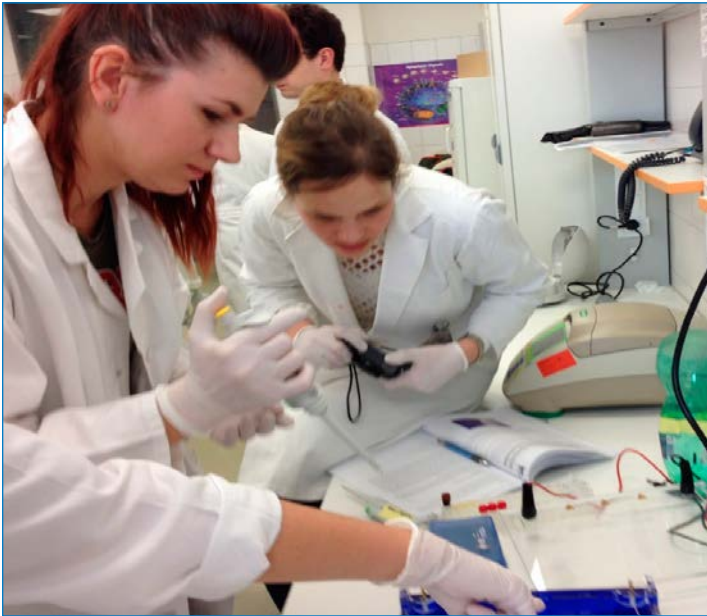
Sample loading on an agarose gel
